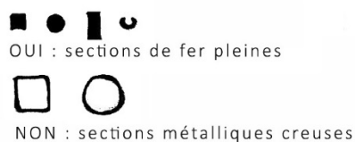
Figure 12 : sections des fers
